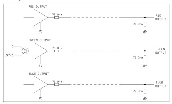
The problem with RGB is that it does use a lot of bandwidth; a better solution is to convert to component video.
