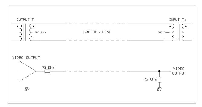
Other than being an unbalanced signal, not a lot different, except for the frequency. Whilst with audio we are typically dealing with a frequency range of 20Hz to 20KHz, more or less, with composite video the frequency is more in the order of 5.5MHz and creates a greater need for due diligence in connection and termination.
