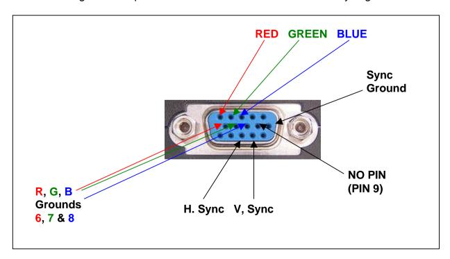
Note that on the above diagram pin 9 is missing. This is the official VGA pin out and whilst all the grounds are on the middle row, these should be kept separate, although they are linked on some equipment along with the 'unused' pin 9.
