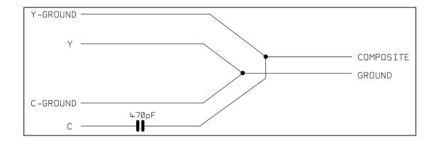
Whilst this can be used in the reverse form to split composite to Y/C, the resultant signal is of very poor quality so it is always best to use an active converter if this is required.
