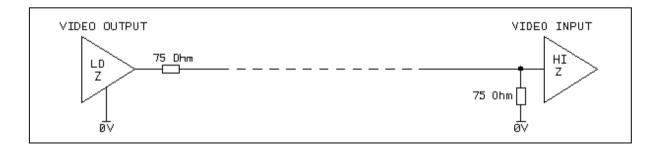
It should be obvious that to achieve a 1Vp-p at the destination, we need a 2V p-p signal to start with. This does though have an advantage if we want to split the signal. In its simplest form we need just two additional resistors to achieve a 3 way Video D/A provide the drive circuit is capable of the current required.
