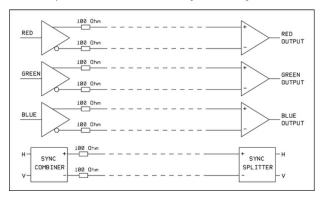
The RGB part of the distribution should look familiar, its just a standard balanced line transmitter and receiver, just optimised for 100 ohm cable. It does use all four pairs of the cable though.
