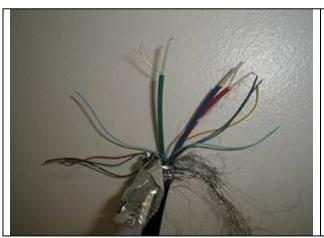
Whilst the use of pre-made VGA to VGA cable may appear attractive from a cost and convenience viewpoint, you get what you pay for. The three 'coax' video cores are not even that, just a centre core and around 6 strands of 'ground' laid by its side and in no way can maintain the 75 oh characteristic impendence. The whole assemble relies on the outer foil covering and loose woven braiding for screening.
