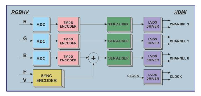
To convert VGA to HDMI we would first need to digitise each pixel for Red, Green and Blue with separate 8 bit ADC's. This would then need converting to 10 bits and TDMS encoding. The encoded bits are now serialised before being sent to the LDVS current drive.
