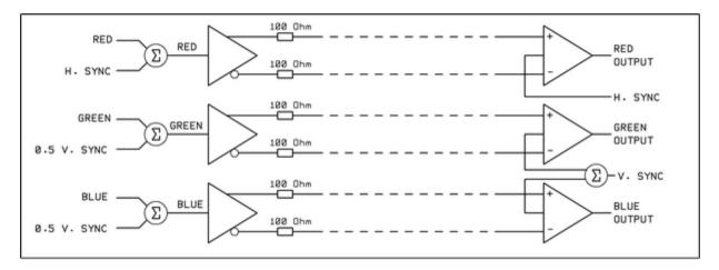
Here we are using the same principle as phantom power to share the syncs across the three colours introduced at the null point of the signal and recovered at the receiver. This leaves us a spare pair for power, audio, control or a combination of all three.
