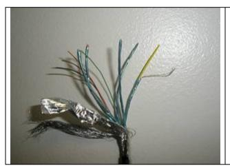
Only suitable for the stated purpose and manufactured of flexibility. You can see that whilst there is an overall foil and braded screen the latter is very open mesh for flexibility. Also have a look at how thin the Video cores are. At least they each have a foil screen and drain cable.
