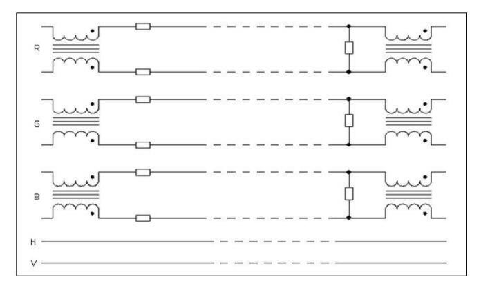
Being a passive circuit the loading upon the drive circuit is at least the same as a normal 75-ohm video load and possibly more when losses due to the impedance change and cable length are taken into account.
