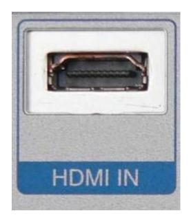
**HDMI Type A plug and Socket**
