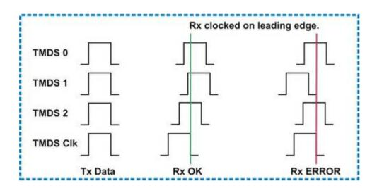
Of course the quality of the cable does have an effect, not so much on the above but the maximum distance you can send the signal before needing a repeater (to reclock the signals).
