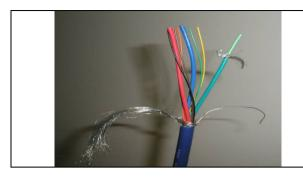
On this cable, costing about 10 times the cost of the previous example, you can see that the video cables are true coax types with individual foil and braded ground. The overall cable assemble has both foil and braded overall screen complete with drain wire.
